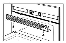
**Step 2:** Remove the front grille by taking out the 2 screws that hold it in place.
